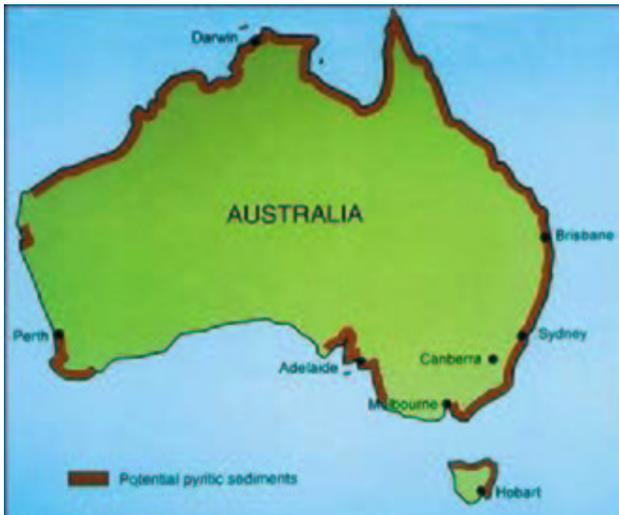
Figure 1. Coastal acid sulphate soils in Australia. (original source, National Strategy for the Management of Coastal Acid Sulphate Soils, January 2000) [deh, 2004].
